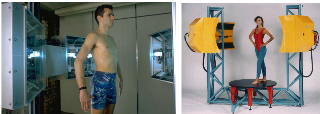
Figure 2. (top) Tecmath/Vitronic/Vitus Pro (The Netherlands). The resolution of the system was 2mm vertically and 1mm horizontally); (bottom) Cyberware WB4 (North America/Italy)
