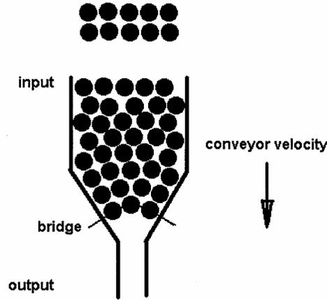
Figure 2. Arch formed from cylindrical components.
