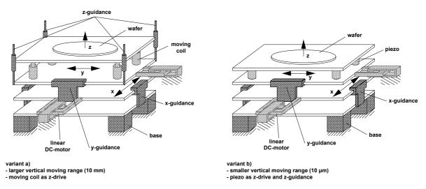
Figure 7. Three coordinate positioning units.
