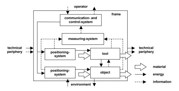
Figure 2. General function structure of nano-positioning machines.
