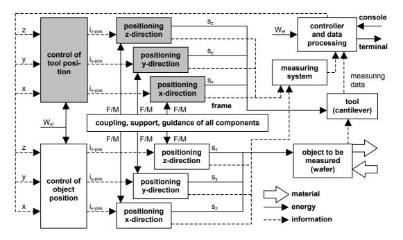
Figure 5. Maximum function structure specified for the wafer inspection by elimination of the shadowed subfunctions.
