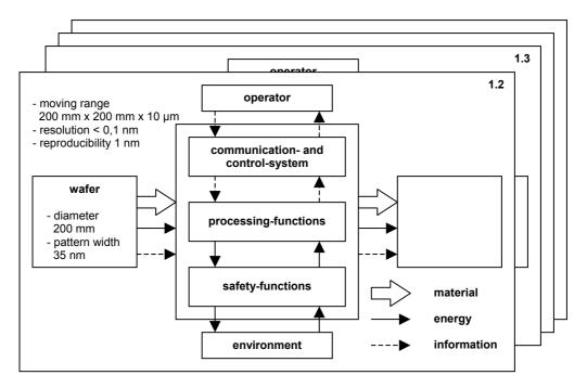
Figure 1. Overall function of a nano-positioning system.
