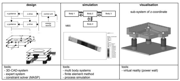
Figure 8. Virtual prototyping in function oriented configuration.
