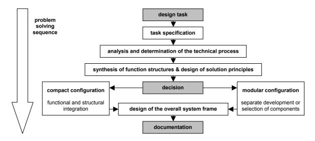
Figure 3. The design process for function-oriented configuration.
