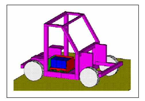
Figure 6. General layout of the battery detachment system.
