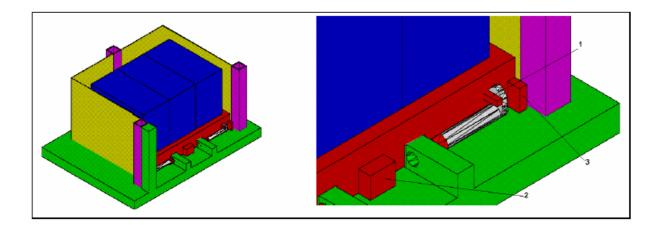
Figure 5. General layout of the battery detachment system and in particular the blocking system, consisting in a stop pin which can be easily operated by any user.
