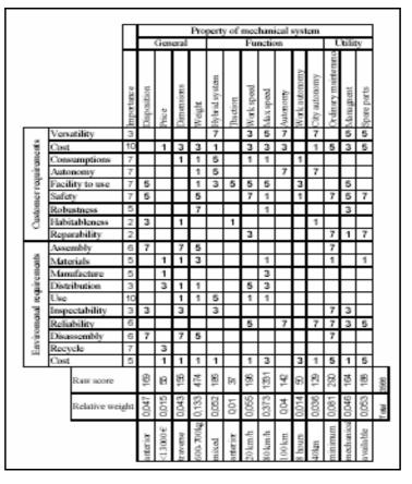
Figure 4. Use of the QFDE matrix in the first phase of the Design Process.
