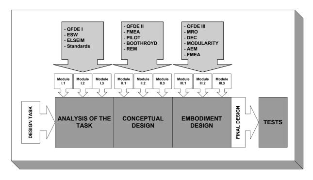
Figure 2. Scheme of the implementation of DFA and DFRR tools within the Design Process (example).
