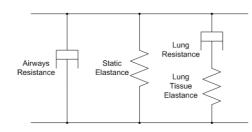
Figure 2 A mechanical diagram, modelling the pulmonary system of dogs
