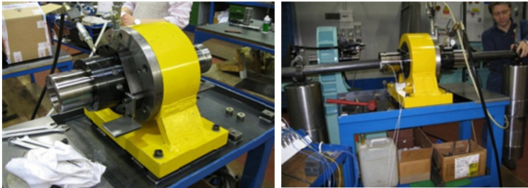
Figure 5. Hydrostatic unit's qualification check
