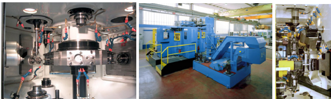
Figure 1. A transfer machine inside: multiple machining units
