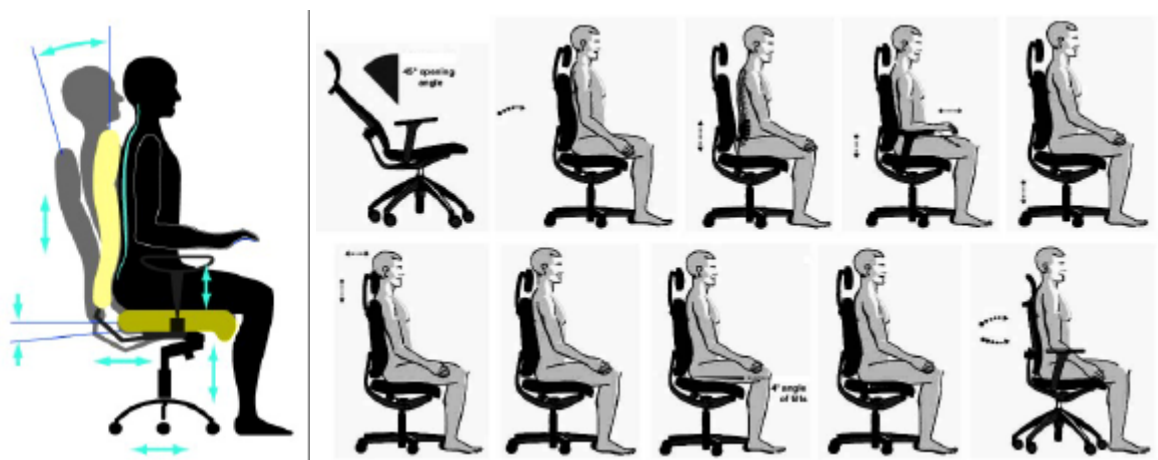
Figure 5. Some of the features that ergonomically designed work chair should have
