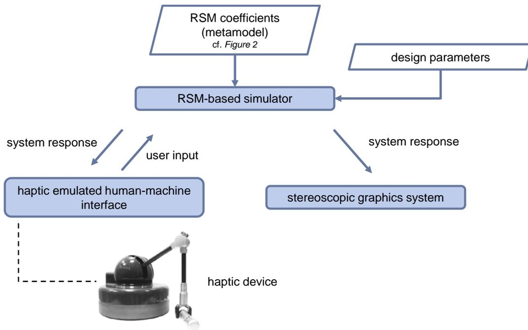
Figure 3. Topology of the simulation system
