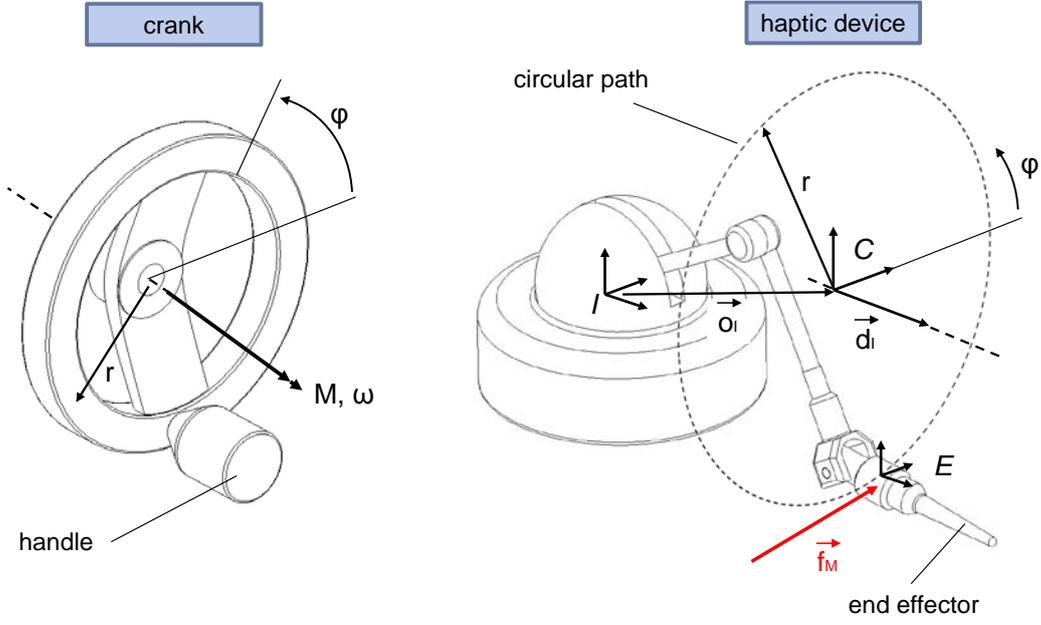
Figure 7. Emulation of a mechanical crank
