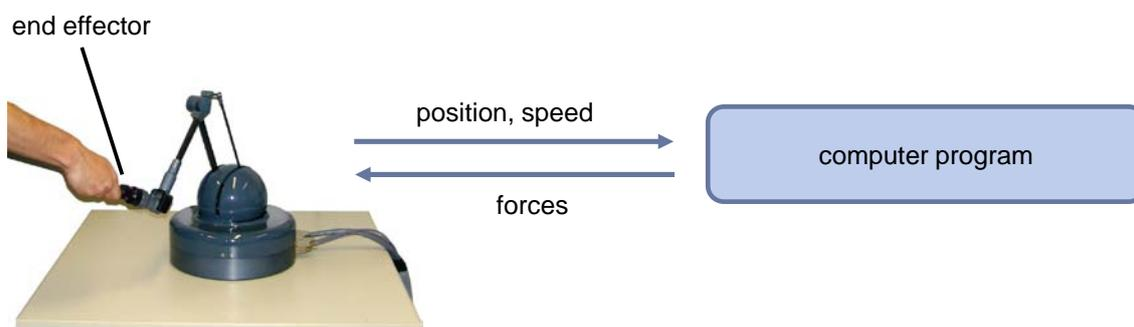
Figure 4. The haptic device and computer interface
