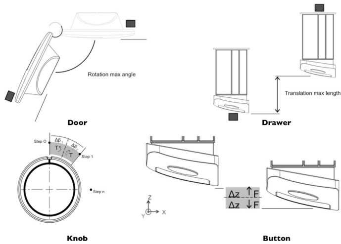
**Figure 4.** Implementation of the four haptic effects.
