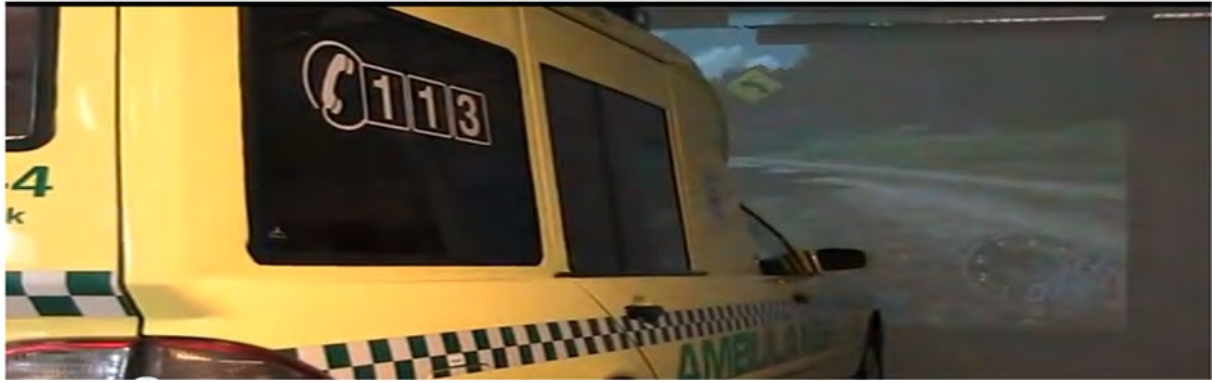
Figure 8. shows an example of the virtual road the ambulance driver had to maneuver the ambulance on
