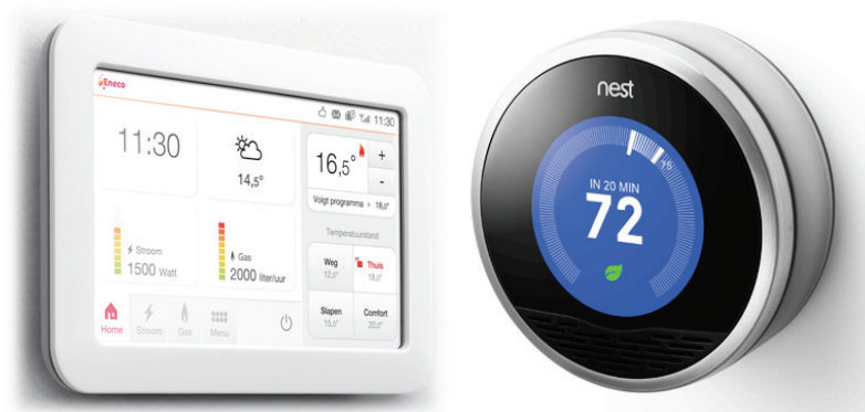
Figure 1. Two smart thermostats, the Toon (left) showing real time energy use and the Nest (right) analyzing user behaviour to automate the heating schedule.
