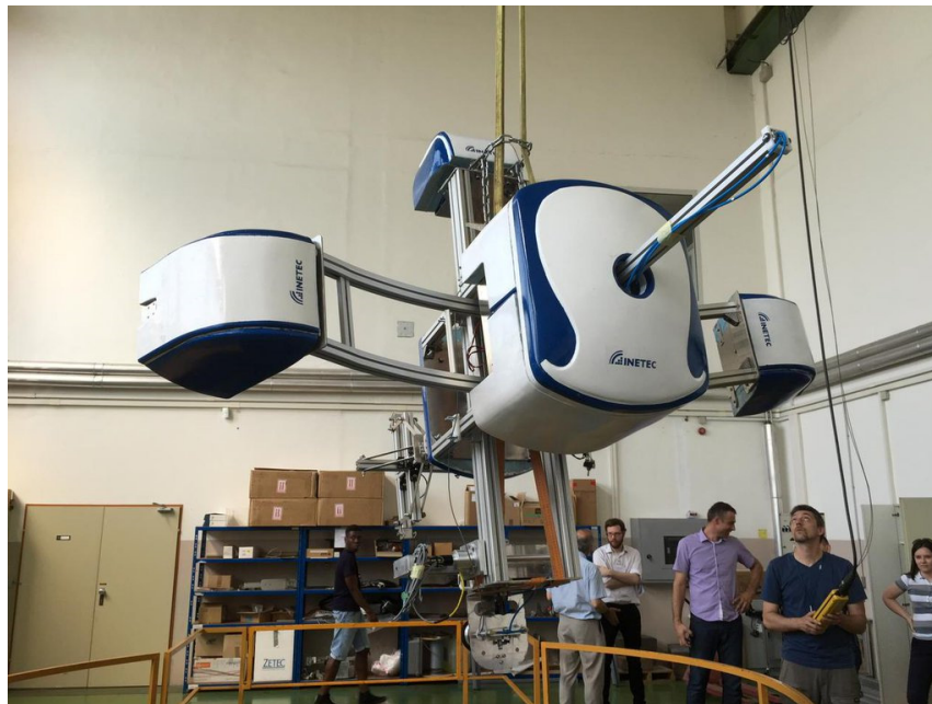
Figure 4. Common 2015 project prototype - robot for inspection of nuclear power plant reactor pressure vessel
