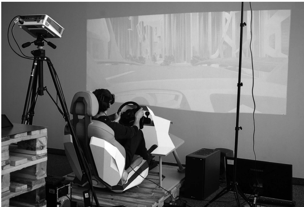
Figure 3. seat box "immersive dynamics" with force-feedback seat, VR glasses and corresponding projection wall
